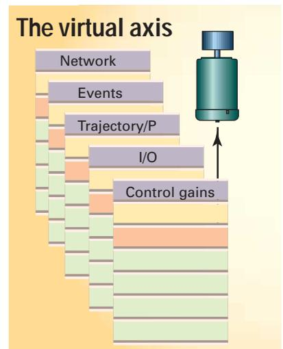
**A register model that captures all relevant information associated with a single motion axis makes it possible for all components in a peer-to-peer network to keep track of each other and work together.**
